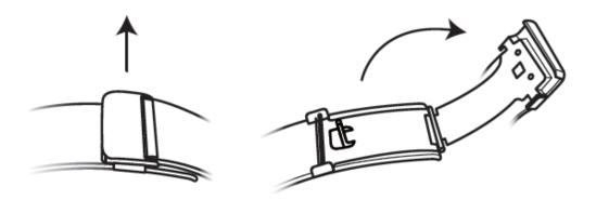
2. Pull the bottom plate upward so it is at a 90° angle with the strap.
