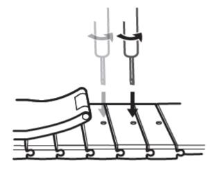
2. Remove a link from both sides of the clasp to make sure the watch face is still centred.
