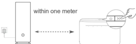
Step 2: When the indicator on the HUAWEI CPE starts to flash, press the **H** button on it. Wait until the indicator on the router shows that the router is connected to the network.
