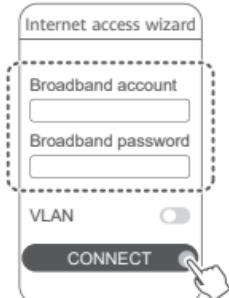
**i** If you need to configure VLAN on your network, contact your broadband carrier to confirm the VLAN parameters, and enable the VLAN switch on the screen.
