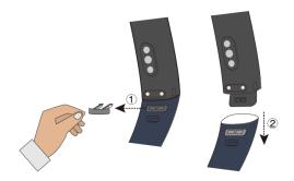
Removal method 2: Remove the fastener from the back of the strap and push the strap from the back of the device to the screen to separate the strap from the device's body.
