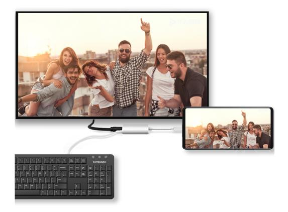
**3** On the external display, set the corresponding HDMI, DP, or MiniDP input as the signal source.
